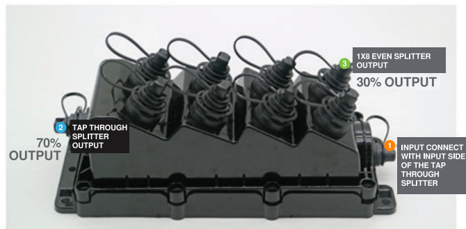
Underterminated 8-port LB-MST 1x2 70/30 coupler with 1x8 splitter (LB-MST-108-70/30)
