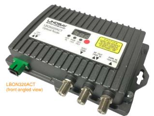
The LBON320ACT device uses an LED display to show the selected channel/wavelength of the ONU. The LED display will also show the optical receive input level in dBm. A pushbutton beside the display allows the user to select the desired wavelength. The LBON320ACT device supports 42/54 MHz, 65/85 MHz and 85/102 MHz frequency splits with the downstream frequency band out to 1218 MHz. The LBON320ACT device series comes standard with Automatic Gain Control (AGC) and burst-mode return lasers.
